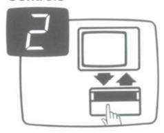
When you press any of the tape transport buttons, the video deck switches on, closes the cassette holder and starts to play, record, rewind, etc., depending upon the button pressed. All controls (except Eject) have a coloured indicator that lights whenever the function is carried out. You can press any tape transport button after any other without pressing the Stop button in between, without harming the cassette or the video deck.
